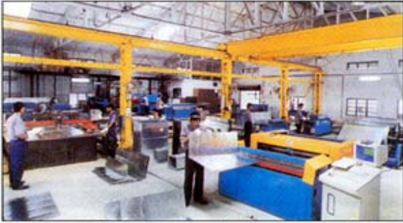
Photo 1 Typical layout of sheet metal profile manufacturing facility for rectangular ducting
